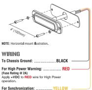
Connect YELLOW wires of all lightheads together for synchronization. (All lightheads should be set to the same pattern)
